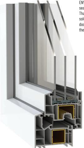
ENVIQ is a modern MD system with an installation depth of 81 mm and a third flexible center seal, offering extended reinforcement chambers to increase the windows' rigidity. Thanks to its optimum profile height, the system provides up to 5% more light than other solutions in its class. Moreover, it includes transition profiles for large sliding and balcony doors and allows the use of bonded glass technology, increasing stability and enabling the creation of larger structures.
